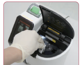
Place the Reagent Cartridges into the chambers.
