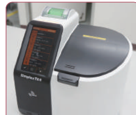
Close the lid and then measurement starts.
