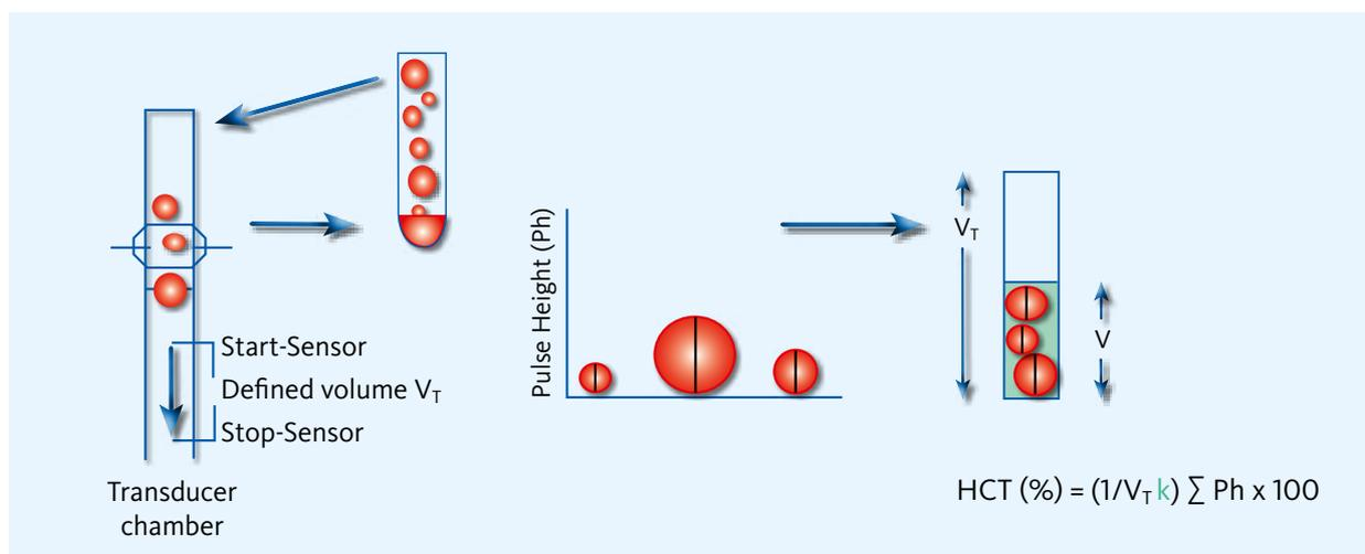
**Fig. 3** Schematic representation of automated HCT measurement using cumulative pulse height detection (for calculation see Fig. 4).
