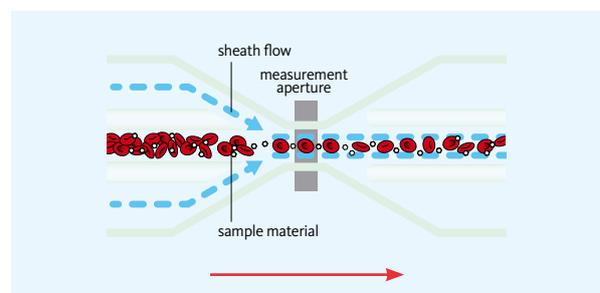
**Fig. 1** Impedance principle with hydrodynamic focusing
